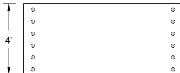
Diagram 3: Single span setup (2 points of attachment)
